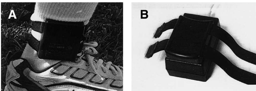
Fig 1. (A) The SAM is attached with 2 elastic straps (left) and is worn on the lateral aspect of the right ankle. (B) Data from the SAM are downloaded to and settings are uploaded from a computer via a dock.
